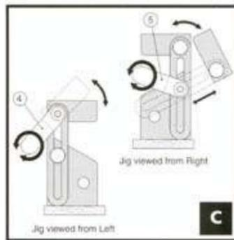
1. Position jig so front edge of **stationary** grindstone is 1/2" (12mm) from back of jig.
