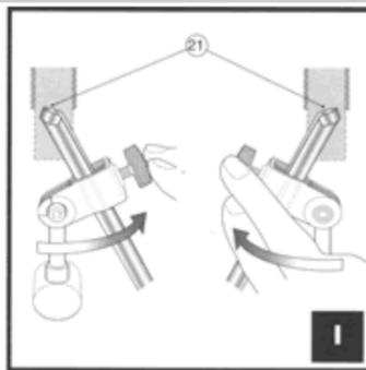
14. Bowl gouges at - 60° bevel angle. Slide gouge into clamp with 2" (50mm) projecting.
