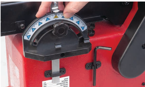
Mitre fence and Hex key storage holders
