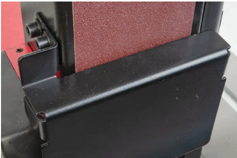
Linisher guard/Workstop, can be used as a work support when the linisher is in the vertical position
